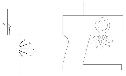
Position a: Top position, for forward direction or run forward in top speed (This function is programmable)
