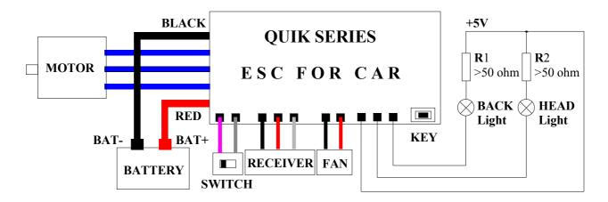
**NOTE:** 1.Only QUIK-60A, 80A and 100A can connect car light (refer to wiring diagram). The resistance of R1 and R2 which limit to current should be greater than 50 ohm, it recommended for  $100\Omega$ , 1/2W resistance of the metal mold.
